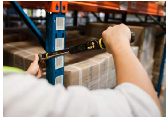
Inspection of Torque Values of Fasteners
