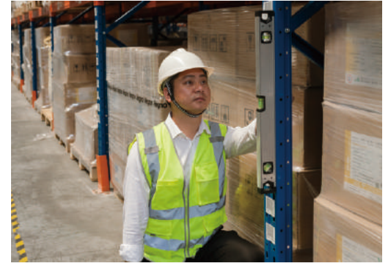
Measurement of Local Deformation
