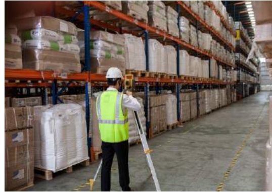
Inspection of Beam Deflection
